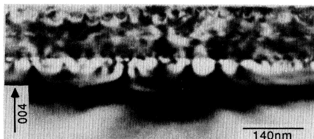
FIG. 2. The low-magnification bright-field image of a Si_{12}/Ge_4 SLS and a Si substrate taken (a) at a 004 Bragg condition, and (b) at a 040 Bragg condition. The appearance and disappearance of dislocations are not due to the g \cdot b effect. These photographs were taken at different places on the specimen.
