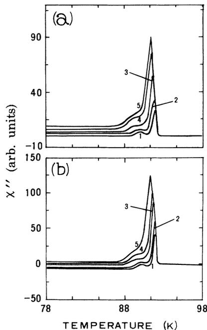
FIG. 3.  $\chi''$  as a function of temperature (a) at a frequency of 137 Hz and (b) at a frequency of 737 Hz in the different ac magnetic-field amplitudes. The magnetic-field amplitudes  $H_0$  corresponding to curves labeled 1, 2, 3, 4, and 5 for 137 Hz are 0.0849, 0.229, 0.399, 0.569, and 1.02 Oe (rms), and for 737 Hz are 0.0425, 0.0849, 0.509, 0.679, and 1.02 Oe (rms), respectively. Curves at 0.170 and 0.340 Oe (rms) for 737 Hz are not shown in (b) for clarity.
