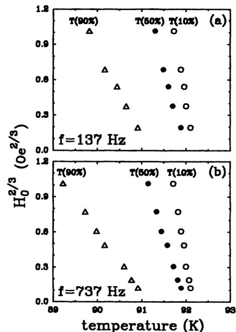
FIG. 2. Temperatures at 10%, 50%, and 90% of the transition in  $\chi'$  vs  $H_0^{2/3}$  (rms); the external ac magnetic-field amplitude (a) at a frequency of 137 Hz, and (b) at a frequency of 737 Hz.
