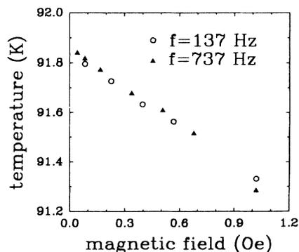
FIG. 5. Temperature at the maximum of the first peak in  $\chi''$  vs  $H_0$  (rms); the external ac magnetic-field amplitude at frequencies of 137 and 737 Hz.
