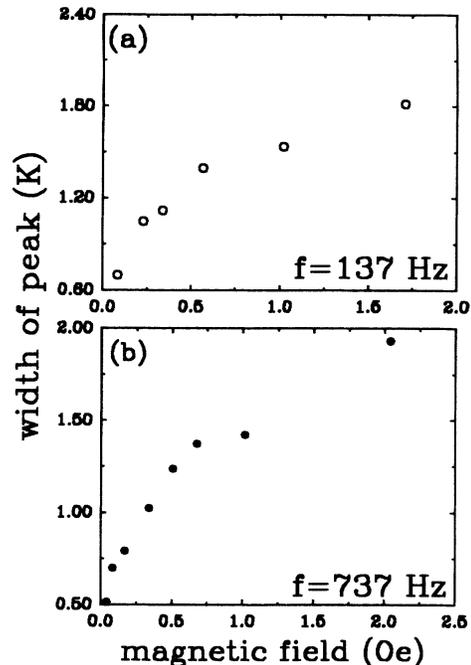
FIG. 4. The width of the first peak in  $\chi''$  vs  $H_0$  (rms); the external ac magnetic-field amplitude (a) at a frequency of 137 Hz and (b) at a frequency of 737 Hz.
