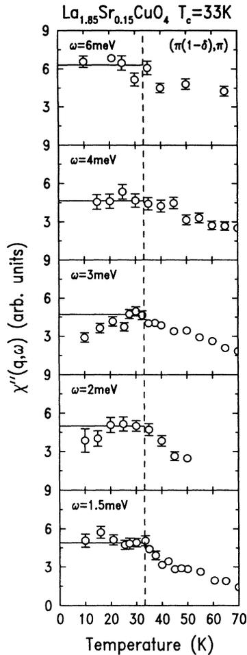
FIG. 4. Temperature dependence of  $\chi''(\mathbf{q}, \omega)$  at 1.5, 2, 3, 4, and 6 meV for  $\mathbf{q} = [\pi(1-\delta), \pi]$ . Corrections for higher-order contamination and instrumental resolution have been made to these data. The solid lines below  $T_c$  are simply constants.
