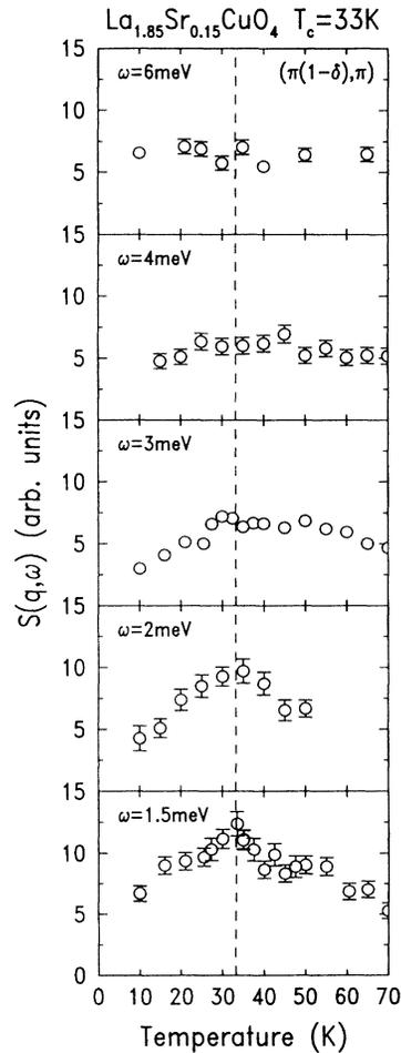
FIG. 3. (a) Temperature dependence of the peak intensity at the  $[\pi(1-\delta), \pi]$  position for energies of 1.5, 2, 3, 4 and 6 meV. Higher-order and resolution corrections have been applied, and smooth, weakly temperature-dependent backgrounds subtracted.
