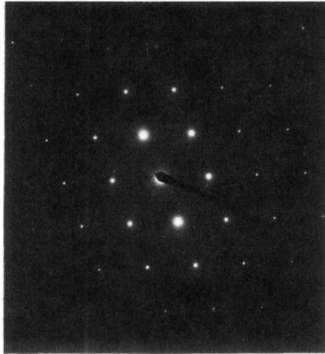
FIG. 6. (431) electron-diffraction pattern of a 1:2:3 crystal obtained from a cross-sectional sample. The c axis of the 1:2:3 phase makes an angle of \sim 86.2^\circ with the plane normal, indicating that the 1:2:3 phase grows with the c axis perpendicular to the traveling direction of the sample.
