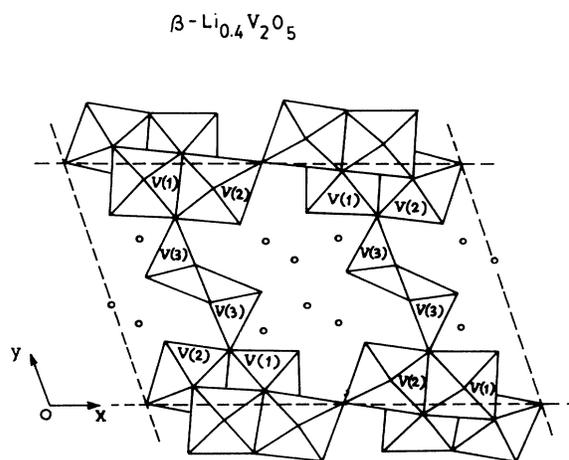
FIG. 1. Crystal structure of lithium  $\beta$  bronze.
