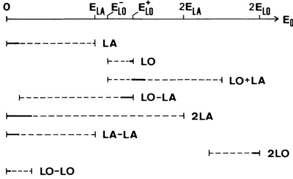
FIG. 1. Schematic diagram showing the possible phonon processes, indicated by bars, against level spacing  $E_0$ . Here,  $E_{LA}$  denotes the maximum LA phonon energy, and  $E_{LO}^-$  and  $E_{LO}^+ = \hbar\omega_{LO}$  are the minimum (zone edge) and maximum (zone center) LO phonon energy, respectively. Efficient carrier relaxation takes place only for energies indicated by thick solid lines.
