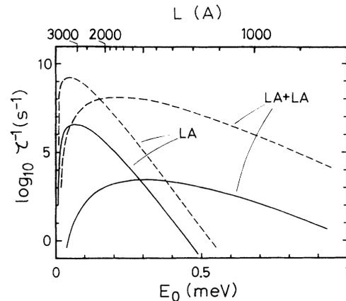
FIG. 3. Calculated electron relaxation rate  $1/\tau$  for small  $E_0$ . The solid curves are for  $T = 0 \text{ K}$ , and the dashed curves are for  $T = 300 \text{ K}$ .
