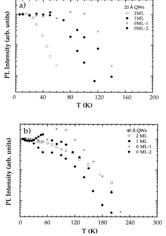
FIG. 3. Temperature dependence of the PL-integrated intensity  $I_L$  of the wells investigated: (a) 20-Å QW's; (b) 40-Å QW's.
