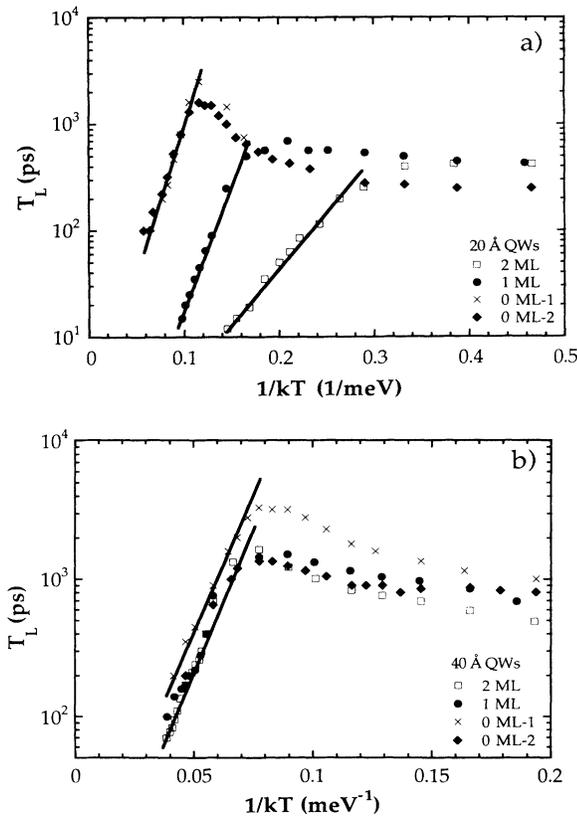
FIG. 5. Arrhenius plot of the PL decay time  $T_L$  versus  $1/KT$  of the wells investigated: (a) 20-Å QW's; (b) 40-Å QW's. The straight lines are the best fits to the high-temperature slopes from which we have extracted the activation energies  $E_A$  reported in Table I. In (b) are reported only the fits to samples 0 ML-1 and 2 ML.
