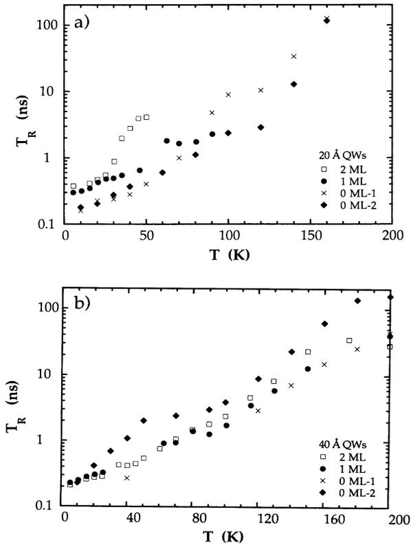
FIG. 4. Temperature dependence of the radiative time constant  $T_R$  of the wells investigated, choosing negligible nonradiative losses at  $T=4$  K [ $T_R(4\text{ K})=T_L(4\text{ K})$ ]: (a) 20-Å QW's; (b) 40-Å QW's.
