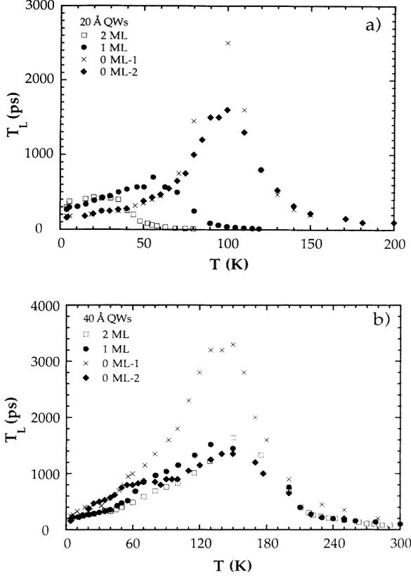
FIG. 2. Temperature dependence of the PL decay time  $T_L$  of the wells investigated: (a) 20-Å QW's; (b) 40-Å QW's.
