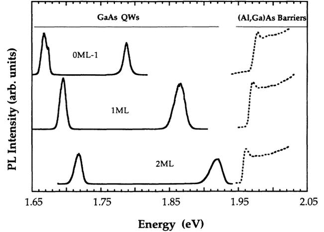
FIG. 1. PL spectra (solid lines) and PLE spectra of 40-Å wells (dotted lines) for the 0 ML-1, 1 ML, and 2 ML samples, respectively. Sample 0 ML-2 shows a similar behavior as 0 ML-1.
