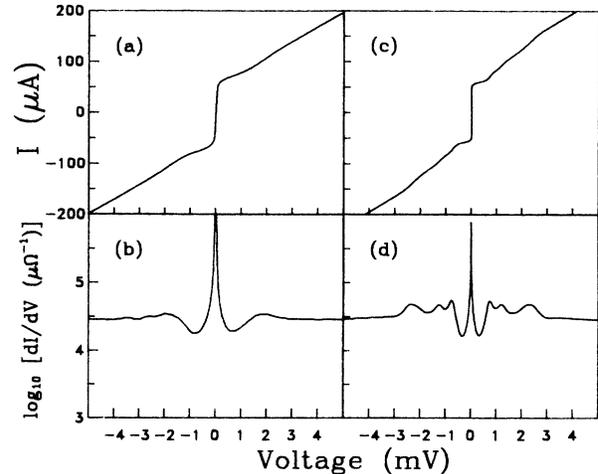
FIG. 3. Experimental curves showing SN Josephson effect and SS Josephson effect. (a) SN  $I$ - $V$  curve; (b) SN differential conductance (log scale); (c) SS  $I$ - $V$  curve; (d) SS differential conductance (log scale). Note the subharmonic structure in SS, which is absent in SN.
