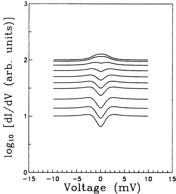
FIG. 2. Model of transition from tunneling to contact using modified BTK model. Note that the, in principle, unknown area would imply an additive constant in the logarithmic plot (but spacing is not arbitrary).
