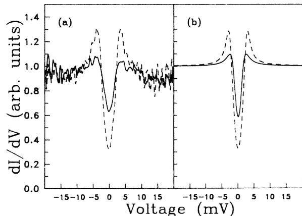
FIG. 4. SN gap compared to SS gap, experimental and theoretical. (a) Experimental differential conductance curves: SS (dotted line), SN (solid line); (b) theoretical differential conductance curves: SS (dotted line), SN (solid line).
