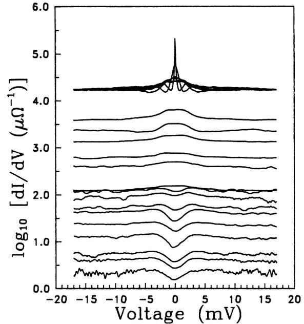
FIG. 1. Experimental conductance curves for Pb (flat) Pt-Rh (tip). Note log vertical scale. Bottom corresponds to high resistance and top to low resistance. Quantum resistance is  $\hbar/2e^2 = 12900 \Omega$  (1.89 in the vertical scale).
