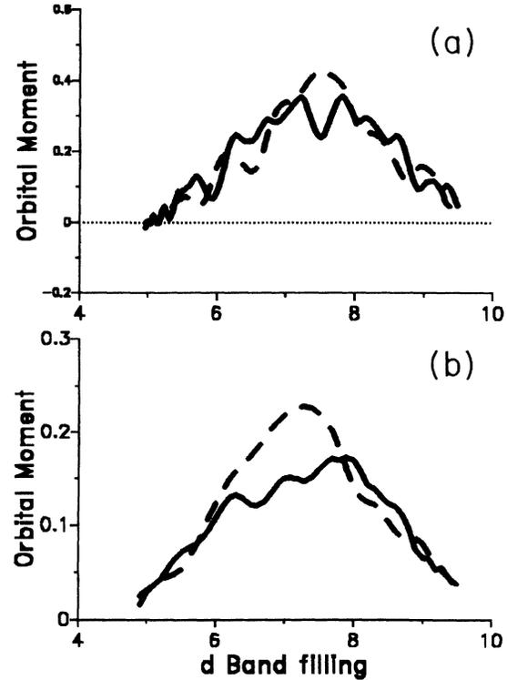
FIG. 2. Magnetic orbital moment per atom (in Bohr magnetons) versus the  $d$ -band filling for (001) monolayer. Full (dashed) line corresponds to the perpendicular (in-plane) direction. (a) Large exchange splitting regime. (b) Small exchange splitting regime.
