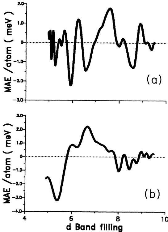
FIG. 1. Magnetic anisotropy energy (MAE) per atom (meV) versus the  $d$ -band filling for (001) monolayer. Negative values correspond to favorable perpendicular direction of the magnetization. (a) Large exchange splitting regime. (b) Small exchange splitting regime.
