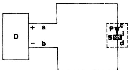
FIG. 4. The schematic diagram of the circuit for the measurements: *D*, digital microvoltmeter, *P*, Pt tip, and *S*, sample.
