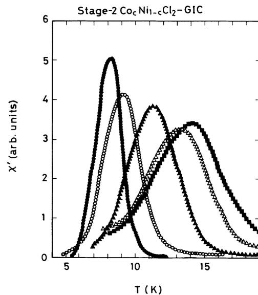
FIG. 2. Real part of ac magnetic susceptibility ( $\chi'$ ) of stage-2  $\text{Co}_c\text{Ni}_{1-c}\text{Cl}_2$  GIC's vs temperature.  $c=0.1$  (■), 0.19 (Δ), 0.40 (▲), 0.63 (○), and 1.0 (●). The ac magnetic field of  $\nu=330$  Hz and  $h=300$  mOe is applied along the  $c$  plane.
