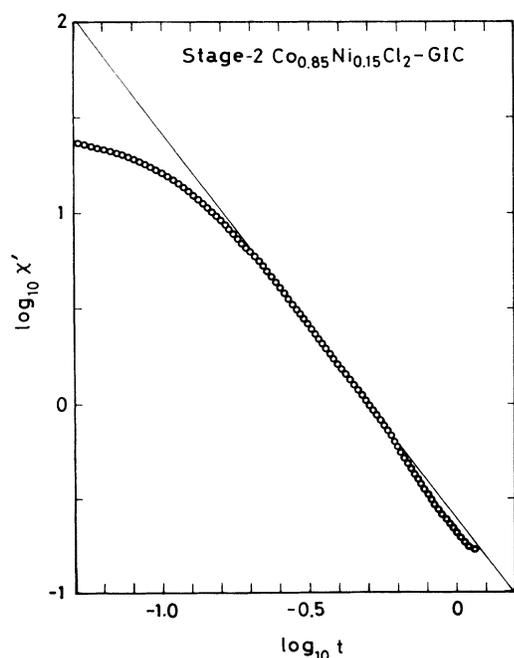
FIG. 4. Log-log plot of  $\chi'$  vs  $t$  ( $t = T/T_c - 1$ ) for stage-2  $\text{Co}_c\text{Ni}_{1-c}\text{Cl}_2$  GIC's with  $c = 0.85$ . The solid line denotes a least-squares fit to the power law with  $\gamma = 2.02$ .
