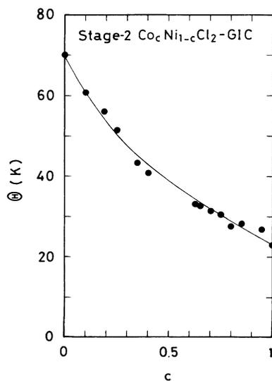
FIG. 1. Curie-Weiss temperature  $\Theta$  vs Co concentration of stage-2  $\text{Co}_c\text{Ni}_{1-c}\text{Cl}_2$  GIC's. The solid line is described by Eq. (14) with  $\Theta(\text{Co-Ni})=p[\Theta(\text{Co})\Theta(\text{Ni})]^{1/2}$  and  $p=1.2$ .
