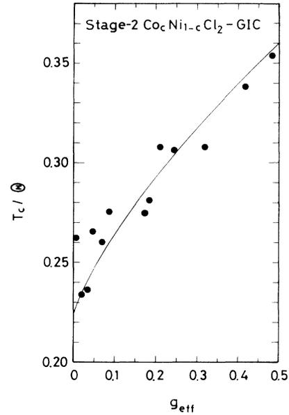
FIG. 7. Plot of  $T_c/\Theta$  as a function of  $XY$  spin anisotropy parameter  $g_{\text{eff}}$  with  $g(\text{Co-Ni})=0.0726$ . The solid line is a result of least-squares fit of the data to Eq. (15) with  $A=0.229$ ,  $B=0.224$ , and  $\phi=1.34$ .
