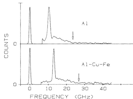
FIG. 1. Sample Brillouin spectra of polycrystalline aluminum (top) and the polycrystalline icosahedral quasicrystal  $\text{Al}_{63.5}\text{Cu}_{24.5}\text{Fe}_{12}$  (bottom) at room temperature. The common free spectral range was 60 GHz. Arrows in both spectra indicate the estimated position of  $k_R v_L$ .
