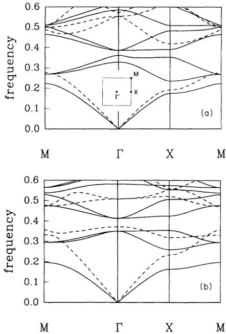
FIG. 1. Photonic band structure of a square lattice of air rods with a filling fraction of 67% in a dielectric material of index 4.25 for  $s$  (—) and  $p$  (---) polarizations. The cross section of the rods is square in (a) and circular in (b). The frequency is given in units of  $2\pi c/a$ , where  $a$  is the length of a unit cell. The inset shows the first Brillouin zone.
