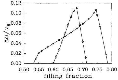
FIG. 2. Ratio of the gap width ( $\Delta\omega$ ) to the midgap frequency ( $\omega_g$ ) as a function of the filling fraction of the air rods in a square lattice of index 4.25. The circles correspond to rods with circular cross section and the squares correspond to rods with square cross section.
