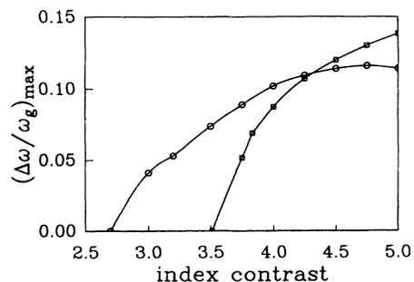
FIG. 3. Maximum gap width to midgap frequency ratio in a square lattice as a function of the index contrast. The circles correspond to rods with circular cross section and the squares correspond to rods with square cross section. The filling fraction of the rods is different for each point of the curves.
