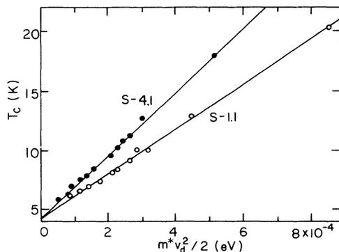
FIG. 2. Effective hot-carrier temperature  $T_c$  as a function of the carrier drift kinetic energy. The temperature values are obtained from the data by using Eq. (8) of the model.
