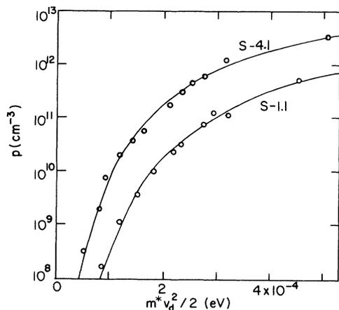
FIG. 1. Hole concentration  $p$  as a function of carrier drift kinetic energy. The curves are calculated from the model as described in the text.
