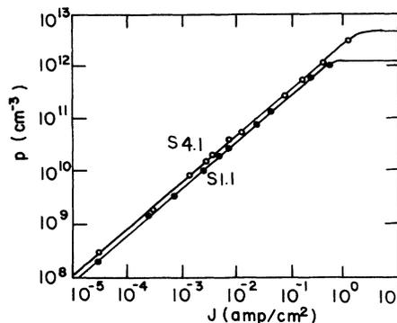
FIG. 3. Hole concentration  $p$  as a function of current density  $J$ .
