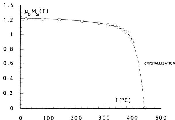
FIG. 1. Spontaneous magnetization as a function of the temperature. Measurements were performed up to temperatures below the crystallization point which, for this composition, is lower than the Curie point of the amorphous state.
