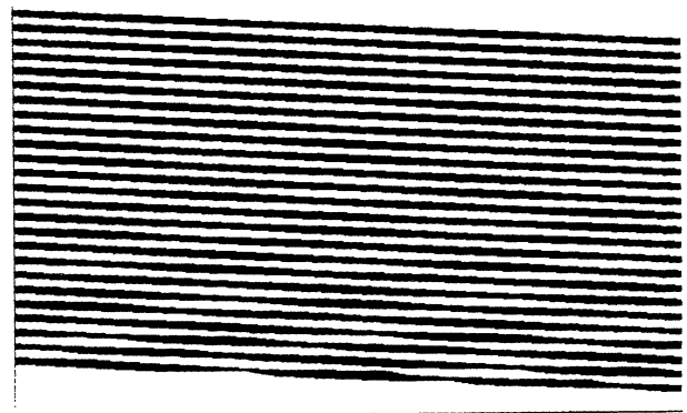
FIG. 4. Numerical simulation of a periodic structure grown on a very nonplanar vicinal surface using lateral step velocities for heteroepitaxy and homoepitaxy corresponding to the center of the terrace-width homogenization regime. The terrace widths quickly evolve to the initial average value, resulting in planar interfaces.
