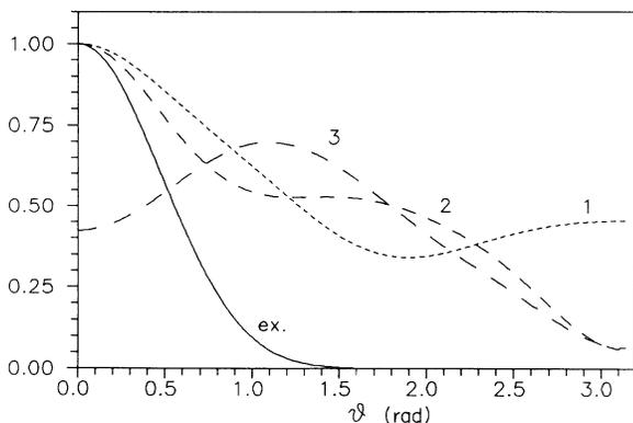
FIG. 2. Angular distribution of the electron density. The function  $\rho_{LM}(\vartheta, \vartheta_h = 0)$  [Eq. (36)] is shown, i.e., the hole resides at the North Pole. The density is normalized to  $n_0(S)$ . Curves 1, 2, and 3 correspond to the three states with  $L = 0$  (Fig. 1), their energies  $E_1 < E_2 < E_3$ . The curve ex. represents a bare exciton.
