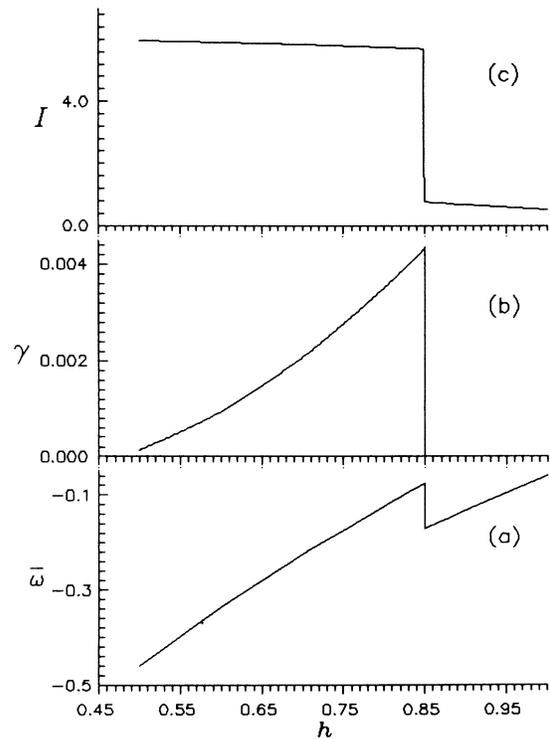
FIG. 5. Basic parameters of the exciton emission band as functions of  $h$ . (a) The position of the band; (b) the bandwidth; (c) the intensity.
