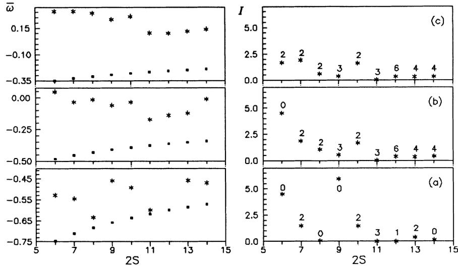
FIG. 6. Exciton emission spectrum vs the inverse filling factor. The left column: the transition frequency; the right column: the transition intensity. Numbers by the asterisks:  $L$  values for the corresponding states. Dressed excitons: asterisks; bare excitons: squares. (a)  $h = 0.5$ ; (b)  $h = 1.0$ ; (c)  $h = 1.5$ .
