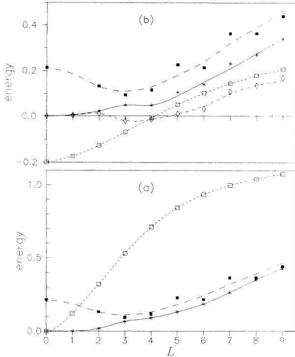
FIG. 3. Energy spectrum of excitons and magnetorotons.  $\square$ : a bare exciton;  $*$ : a dressed exciton;  $\blacksquare$ : magnetorotons. The curves are only guides for the eye. (a) Symmetric system; (b) nonsymmetric system,  $h = 0.5$ , in the latter case the MR energy is plotted from the bottom of the spectrum of a dressed exciton. By diamonds  $\diamond$  the dispersion law of a dressed exciton is shown for  $h = 1.0$ .
