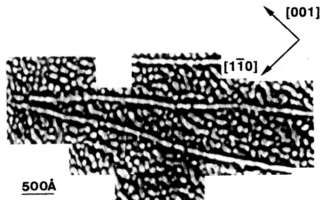
FIG. 5. A mosaic of images taken after 4 ML Ge deposition at 420^\circ\text{C} showing preferential island coalescence along step edges.
