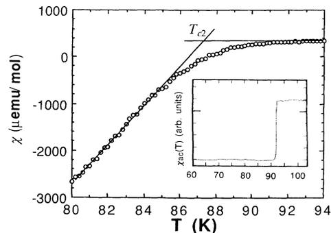
FIG. 1. Temperature dependence of the magnetic susceptibility  $\chi(T)$ , measured in an external field  $H = 50$  kOe parallel to the  $c$  axis of the crystal. The solid lines represent the linear approximation procedure to estimate the nucleation temperature  $T_{c2}$ . The normal-state susceptibility is  $\chi_n \approx 330$   $\mu\text{emu/mol}$ . The inductively measured transition to superconductivity in a field of a few Oersted is shown in the inset.
