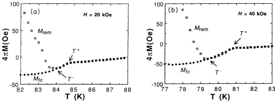
FIG. 2. (a) and (b) Representative  $M_{\text{rem}}(T)$  and  $M_{\text{fc}}(T)$  curves collected using a  $\text{YBa}_2\text{Cu}_3\text{O}_7$  single crystal for external fields  $H$  parallel to the  $c$  axis. The magnetization values  $M$  have been calculated by the software of the magnetometer and do not necessarily represent the true values of  $M$ , namely at temperatures below  $T^*$  (see text). The temperatures  $T'$  and  $T^*$  (see text) are indicated by arrows.
