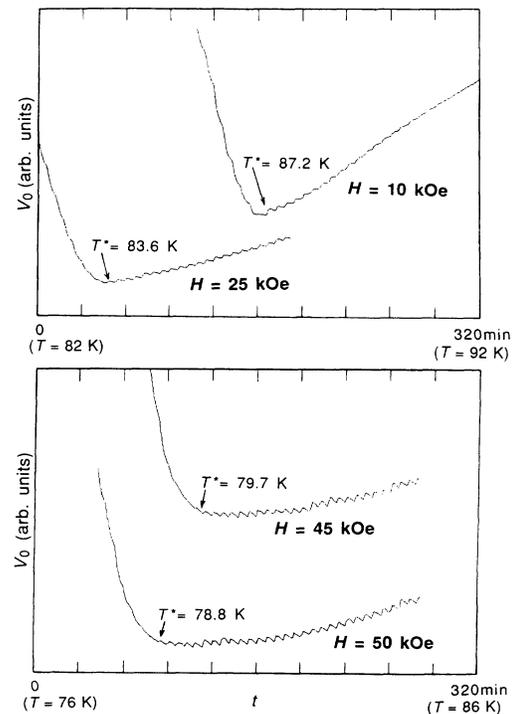
FIG. 5. Typically observed  $V_0(t)$  characteristics. The signal  $V_0$  is a measure of the relative change  $\Delta M$  of the magnetization  $M$  of the sample, although  $V_0$  is not proportional to  $M$  (see text). The  $V_0(t)$  curves include a significant voltage-vs-time drift of the SQUID setup, which does not originate from the sample.
