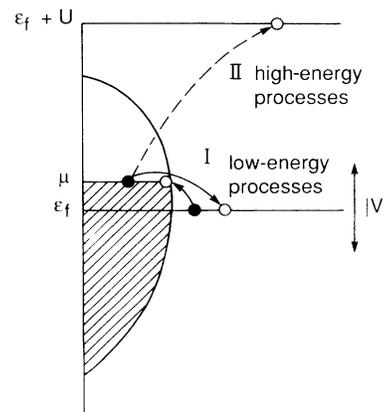
FIG. 1. Schematic representation of the mixing (hybridization) processes and their division into low- and high-energy parts. The former involves only empty and singly occupied atomic level configurations, while the latter takes place via double occupancies in either initial or final states.
