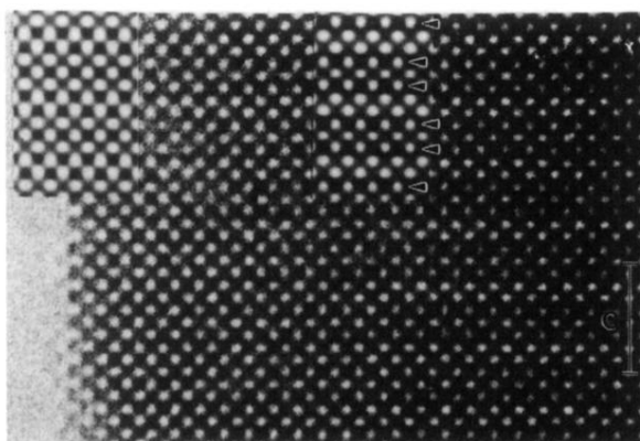
FIG. 4. [110] micrograph of \text{Ba}_3\text{Pb}_2\text{O}_7 . Arrows point to the Pb atom columns. Calculated images at a defocus of -40 nm and thicknesses of 2 nm (left) and 6 nm (right) are given as insets.
