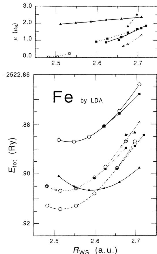
FIG. 1. Total energy  $E_{tot}$  and magnetic moment  $\mu$  of Fe as a function of the Wigner-Seitz radius  $R_{WS}$ , calculated by the LDA of Ceperley and Alder. The solid curve corresponds to the bcc, the dotted to the fcc, and the dashed to the hcp. The circles indicate NM, the triangles FM, and the squares AF, and the filled (open) symbols are for the high-spin (low-spin) state solutions of the corresponding magnetic phase.
