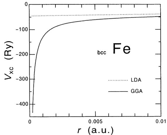
FIG. 3. Comparison of the exchange-correlation potential  $V_{\text{xc}}$  by the GGA with that by the LDA for the majority spin of the bcc Fe. The  $-1/r$  divergence of the GGA exchange-correlation potential is clearly observed and makes a striking contrast to the rather flat behavior of the LDA potential.
