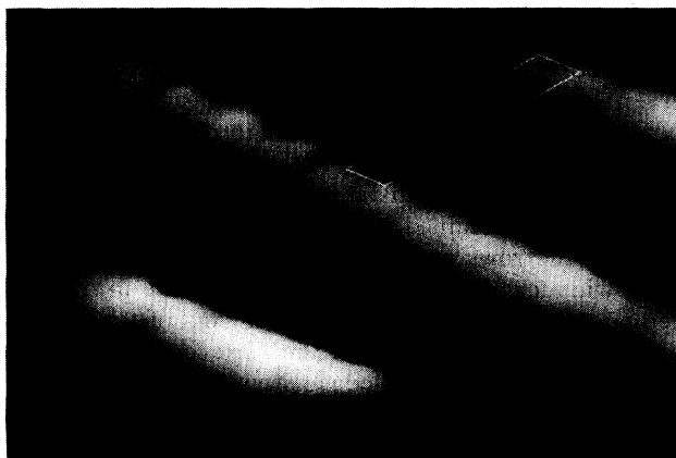
FIG. 2. A 30 \times 40 \text{ \AA}^2 constant-height image of the planar \text{TiO}_2(100)1 \times 3 surface, with the tip stabilized at +2 \text{ V} sample bias and 0.2 \text{ nA} tunneling current before disengaging the feedback loop. The image, in which the rows lie parallel to the [001] direction, is displayed as a tilted, three-dimensional figure for ease of viewing. The 1 \times 3 unit cell is marked on the image which terminates in structure along the rows which we associate with Ti atom positions. The length scales have not been corrected.
