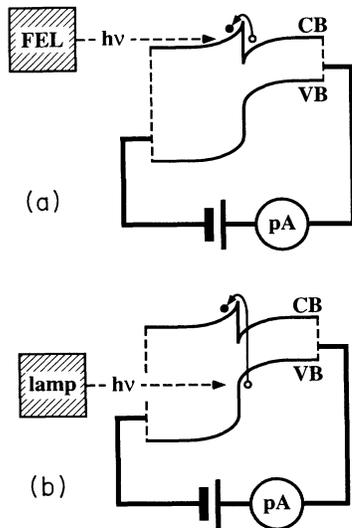
FIG. 1. Simplified schemes of our experiments. (a) Free-electron-laser (FEL) optical pumping experiment, where the pumping across the conduction-band (CB) discontinuity is detected by amplifying and measuring the external current it produces. (b) Similar experiment with a conventional photon source, which gives pumping from the top of the valence band (VB) in one material to the bottom of the CB in the other.
