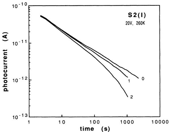
FIG. 8. Effect of bias illumination (BI) on the LTPD in  $\alpha$ -Si:H. The results were obtained for sample S2 in an intermediate Staebler-Wronski state ( $I$  state). Curve 0: without BI; curves 1 and 2: with BI. See the text for details.
