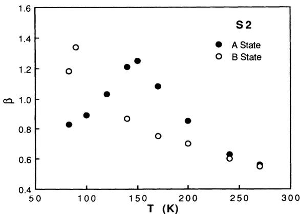
FIG. 5. Effect of light soaking on the decay exponent  $\beta$  for sample S2. Values of  $\beta$  between  $\sim 100$  and  $\sim 150$  K are missing in the *B* state (see the text for details). *A*: annealed state; *B*: light-soaked state.
