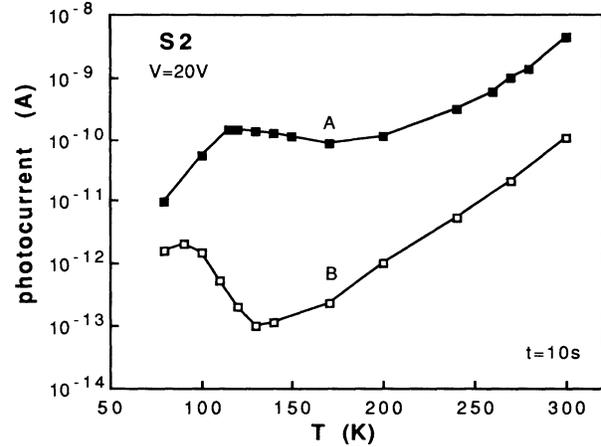
FIG. 6. Effect of light soaking on the photocurrent remaining in sample S2 10 sec after termination of the steady-state illumination. *A*: annealed state; *B*: light-soaked state.
