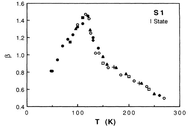
FIG. 3. Temperature dependence of the power-law-decay exponent  $\beta$  for sample S1 in an intermediate Staebler-Wronski state (*I* state). A given symbol represents the values measured in the same run, i.e., without letting the sample return fully to thermal equilibrium between the decay measurements at different temperatures.
