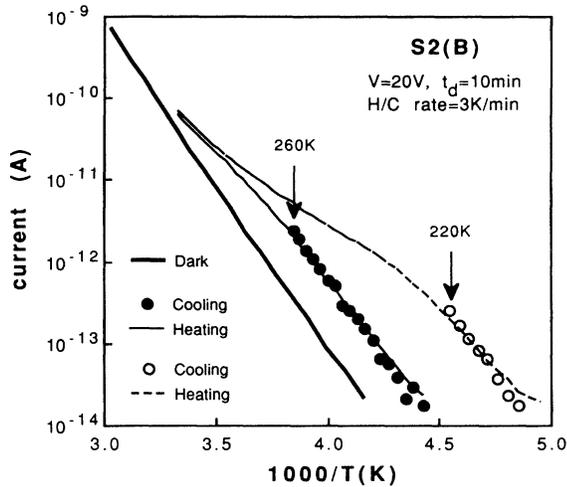
FIG. 7. Total current of sample S2 in the light-soaked state during cooling and heating after the sample was illuminated at the temperatures indicated and after a 10-min delay period. The cooling and heating rate was 3 K/min.
