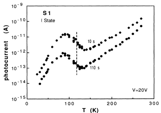
FIG. 4. Temperature dependence of the photocurrents remaining at 10 and 110 sec after termination of the steady-state illumination for sample S1 in an intermediate Staebler-Wronski state (*I* state). The dashed line indicates the temperature at which the peak in the temperature dependence of  $\beta$  appears.
