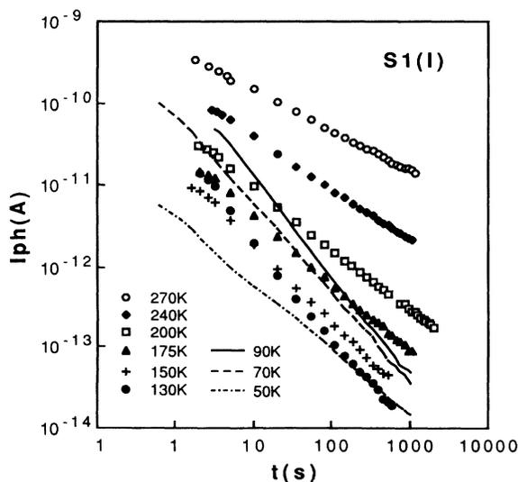
FIG. 2. Limiting power-law decays of photocurrent at various temperatures for sample S1 in an intermediate Staebler-Wronski state (*I* state).
