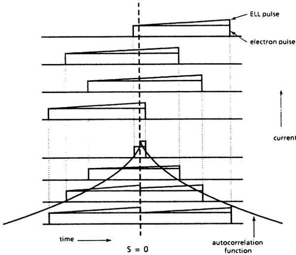
FIG. 3. Current pulses for ELL carriers and electrons.
