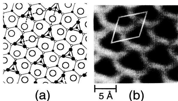
FIG. 2. (a) A diagram of the HCT model for the  $\sqrt{3}\times\sqrt{3}$  surface, drawn to the same scale as (b) a filled-state image of this surface. The Si trimers in the HCT structure are shown as solid circles and heavy triangles. The Ag atoms are large open circles. One unit cell is outlined by a dashed line.
