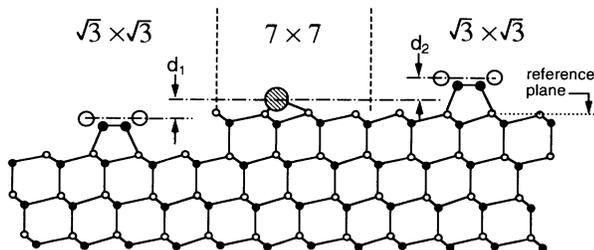
FIG. 4. Schematic view of the two types of boundaries between the  $7\times 7$  structure and the HCT model for the Ag/Si- $\sqrt{3}\times\sqrt{3}$  structure.
