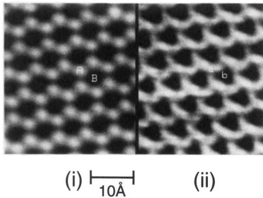
FIG. 1. A pair of images of the  $\text{Ag/Si(111)-}\sqrt{3}\times\sqrt{3}$  structure, showing (i) the empty states and (ii) the filled states.  $A$  and  $a$  mark the position of one of the empty-state maxima in both images.  $B$  and  $b$  mark corresponding minima in both images.
