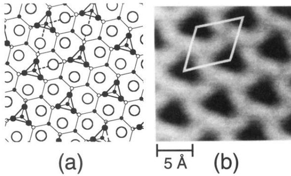
FIG. 2. (a) A diagram of the HCT model for the  $\sqrt{3} \times \sqrt{3}$  surface, drawn to the same scale as (b) a filled-state image of this surface. The Si trimers in the HCT structure are shown as solid circles and heavy triangles. The Ag atoms are large open circles. One unit cell is outlined by a dashed line.
