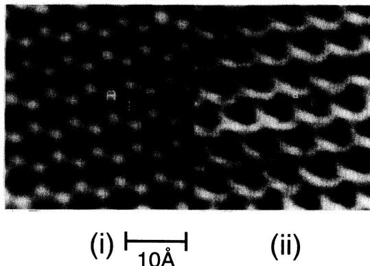
FIG. 1. A pair of images of the Ag/Si(111)- $\sqrt{3}\times\sqrt{3}$  structure, showing (i) the empty states and (ii) the filled states.  $A$  and  $a$  mark the position of one of the empty-state maxima in both images.  $B$  and  $b$  mark corresponding minima in both images.
