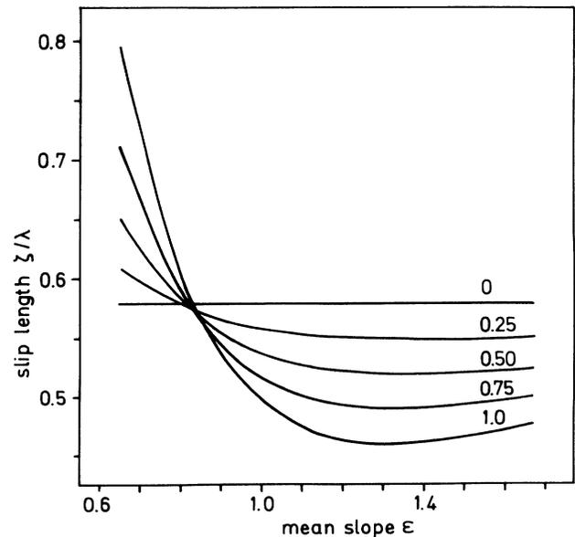
FIG. 2. Slip length  $\zeta$  as function of the mean slope  $\varepsilon$  for a Gaussian-shaped roughness and for different portions  $\rho = 0, 0.25, 0.5, 0.75, 1.0$  of elastic scattering.
