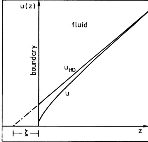
FIG. 1. Definition of the slip length  $\zeta$  for Couette flow.
