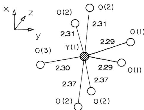
FIG. 8. Environment of the Y(1) atom in  $Y_2BaCuO_5$  (Ref. 3). The interatomic distances are in units of Å.
