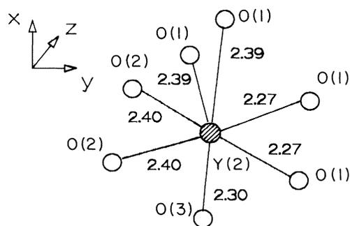
FIG. 7. Environment of the Y(2) atom in  $Y_2BaCuO_5$  (Ref. 3). The interatomic distances are in units of Å.
