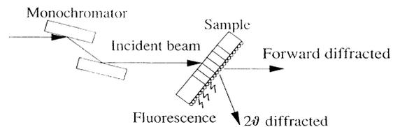
FIG. 1. Schematic layout of the experiment. The incident beam is subjected to the anomalous transmission effect due to the large thickness of the substrate. Only the wave field that has a weak interaction with the substrate can reach the exit face and excite the adsorbate.
