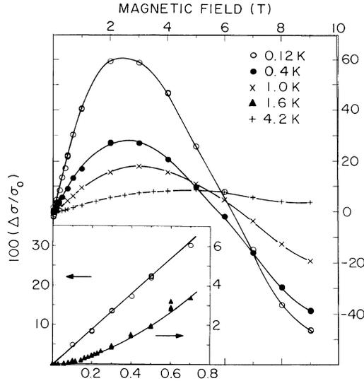
FIG. 1. The longitudinal magnetoconductance,  $\Delta\sigma/\sigma_0 = [\sigma(H) - \sigma(0)]/\sigma(0)$ , of compensated *n*-type CdSe with net dopant concentration  $N_D - N_A = 2.25 \times 10^{17} \text{ cm}^{-3}$  (sample 4) plotted as a function of magnetic field at various temperatures, as labeled. The lines are drawn to guide the eye. The inset shows the behavior in small magnetic field at two different temperatures.
