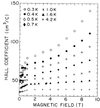
FIG. 2. The Hall coefficient  $R_H$  of compensated *n*-type CdSe with net dopant concentration  $N_D - N_A = 2.25 \times 10^{17} \text{ cm}^{-3}$  (sample 4) plotted as a function of magnetic field at various temperatures, as labeled.
