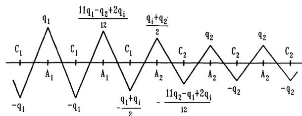
FIG. 1. Charge redistribution around the interface for the zero-dipole condition for a system where the constituents share neither common anion nor cation.  $q_1$ ,  $q_2$ , and  $q_i$  are, respectively, the bulk charges of the barrier, the well, and of the interface.
