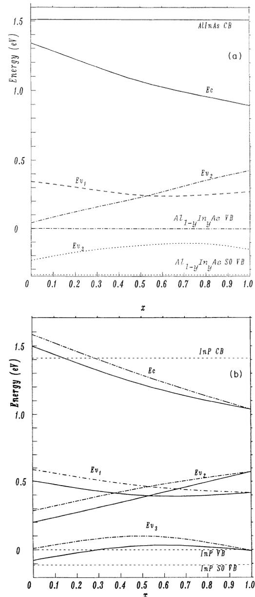
FIG. 2. Band alignments of (a)  $\text{Ga}_{1-x}\text{In}_x\text{As}/\text{Al}_{0.48}\text{In}_{0.52}\text{As}$  and (b)  $\text{Ga}_{1-x}\text{In}_x\text{As}/\text{InP}$  systems; for this latter system, dotted-dashed curves correspond to  $\text{Ga}_{1-x}\text{In}_x\text{P}$  interface, solid curves to an InAs interface, and dashed curves indicate the InP band edges.
