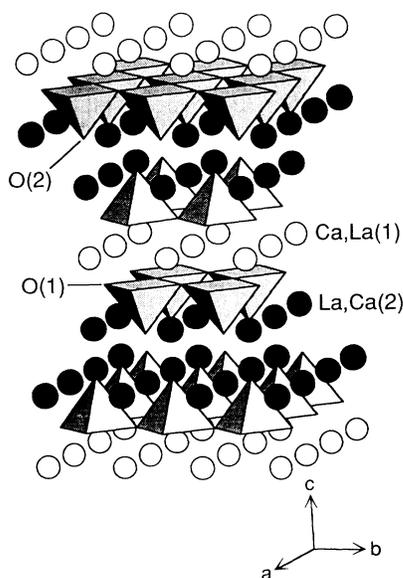
FIG. 1. Crystal structure of  $\text{La}_{2-x}\text{Ca}_{1+x}\text{Cu}_2\text{O}_6$ . The  $[\text{CuO}_5]$  pyramidal planes are the electrically active components.
