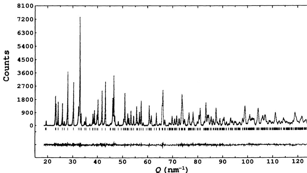
FIG. 4. Rietveld refinement patterns for superconducting  $\text{La}_{1.82}\text{Ca}_{1.18}\text{Cu}_2\text{O}_{6+\delta}$  plotted against  $Q$  ( $=2\pi/d$ ). The background is subtracted. Plus marks show observed neutron-diffraction intensities, and the solid line represents calculated intensities. The curve at the bottom shows the difference between the observed and calculated intensities in the same scale.
