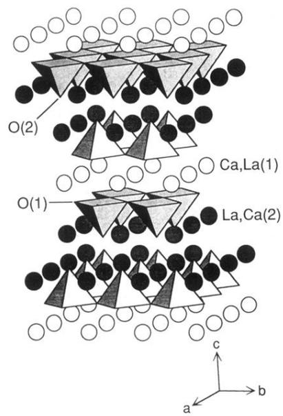
**FIG. 1.** Crystal structure of  $\text{La}_{2-x}\text{Ca}_{1+x}\text{Cu}_2\text{O}_6$ . The  $[\text{CuO}_3]$  pyramidal planes are the electrically active components.
