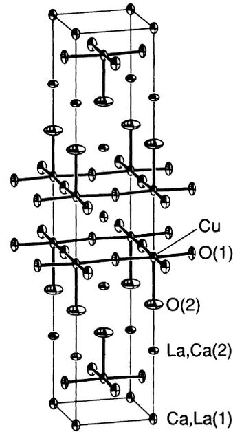
FIG. 5. ORTEP-II drawing of superconducting  $\text{La}_{1.82}\text{Ca}_{1.18}\text{Cu}_2\text{O}_{6+\delta}$ . The thermal ellipsoids are drawn as 95% probability surfaces. Cu and O atoms are connected with bonds.
