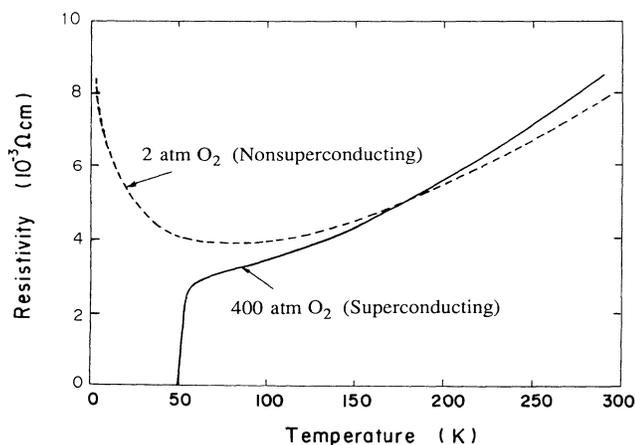
FIG. 2. Electrical resistivity vs temperature for superconducting and nonsuperconducting  $\text{La}_{1.82}\text{Ca}_{1.18}\text{Cu}_2\text{O}_{6\pm\delta}$ .
