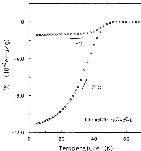
FIG. 3. Magnetic susceptibility vs temperature for superconducting  $\text{La}_{1.82}\text{Ca}_{1.18}\text{Cu}_2\text{O}_{6+\delta}$ . Susceptibility was measured in zero-field-cooling (ZFC) and field-cooling (FC) conditions.
