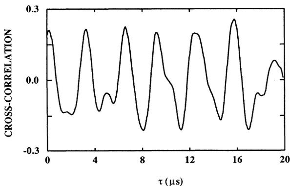
FIG. 6. Correlation of the velocity oscillations with the surface profile in a region 20 mm after transition is shown in this graph of the cross-correlation function  $\Sigma, A(t + \tau)V(t)$ , where  $A(t)$  and  $V(t)$  are, respectively, the surface height and fluctuating part of the velocity, normalized by their rms values, and  $\tau$  is the delay time.
