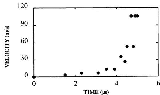
FIG. 8. Velocity of the crack as a function of time during the first 5  $\mu$ s (0.1 mm) of fracture. The data were measured on a sample having an initial crack length of 67 mm, which was 34% of the initial sample size in the  $x$  direction. The initial motion is seen to result from smooth acceleration from rest and not by a discontinuous jump to a finite velocity.
