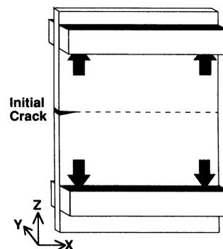
FIG. 1. Schematic representation of the method of loading used in the experiments: Stress was applied in the  $z$  direction (arrows) to the undersides of strips bonded onto the upper and lower edges of the plate. The dashed line shows the crack's direction of propagation starting from an imposed initial crack.
