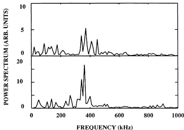
FIG. 9. Power spectra of surface height (see Ref. 30). The upper spectrum was obtained for the surface created in the  $100 \mu\text{s}$  immediately following the onset of oscillations, the lower for the surface created in the subsequent  $100 \mu\text{s}$ . Although the mean velocity of the crack increases by over 60%, the frequency of oscillation remains constant.
