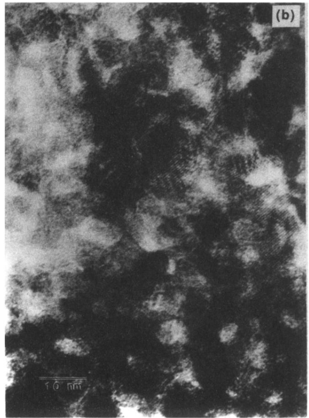
FIG. 8. TEM micrographs of \text{Fe}_{66}\text{Co}_{18}\text{Si}_1\text{B}_{15} after (a) 8 h and (b) 25 h of milling.
