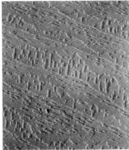
FIG. 5. A STM image over an area of 3500 \times 4000 \text{ \AA}^2 of Si(100) dosed with 3.3-L disilane at 455^\circ\text{C} . The sample bias is -2 \text{ V} . Terrace heights increase from the lower left of the micrograph toward the upper right.
