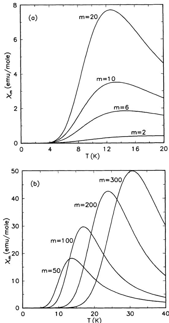
FIG. 2. Theoretical susceptibility vs temperature for a gas of noninteracting, Fermi-like  $m$ -fold spin clusters in an applied field of 1000 Oe. (a)  $m = 2, 6, 10, 20$ . (b)  $m = 50, 100, 200, 300$ .
