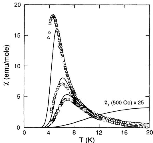
FIG. 1. Susceptibility vs temperature for a single crystal of FeTAC, with the applied field along the easy axis, for fields of 500 (Δ), 1000 (○), and 1500 (□) Oe. Theoretical fits of the exact susceptibility for the Ising chain ferromagnet with *J*/*k* = 17.5 K, *g* = 7.5 are shown as solid lines. The curve labeled  $\chi_1(500 \text{ Oe}) \times 25$  is for single-spin reversals, and is multiplied by a factor of 25.
