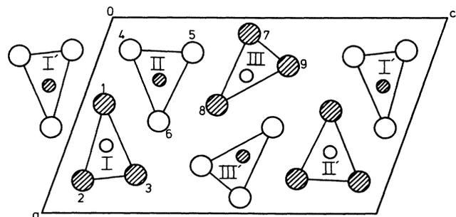
FIG. 1. Projection along  $b$  of a part of the structure of one unit cell thickness. Small and large circles denote Nb and Se atoms, respectively. Open circles correspond to atoms at  $z = \frac{1}{4}$ ; hatched circles represent atoms at  $z = \frac{3}{4}$ . Arabic numbers correspond to the Se atoms in Table I. Primed numbers indicate symmetry equivalent columns.
