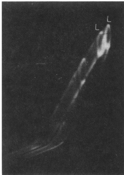
FIG. 12. A hysteresis loop traced at 100 KHz. Note the localized hysteresis loops marked L .
