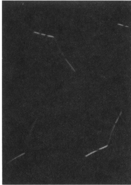
FIG. 18. A switching transient observed in the \text{KNbO}_3 single crystal containing cooperatively ordered impurity dipoles.
