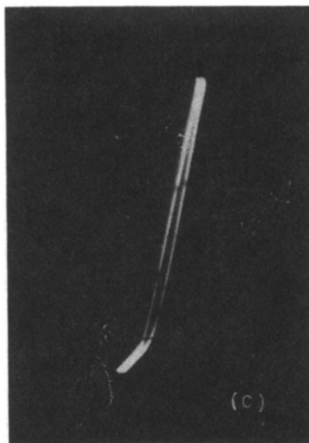
FIG. 13. The hysteresis loops traced at various tracing frequencies (a) 10, (b) 50, and (c) 70 KHz.
