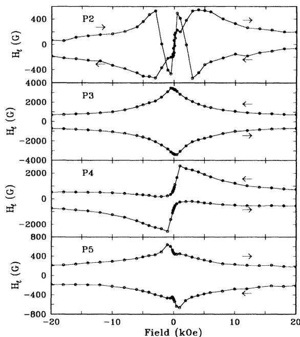
FIG. 3. Local-field hysteresses near zero external field at 4.3 K. The suppression of the local field and its variation with the position of the Hall probe is apparent.
