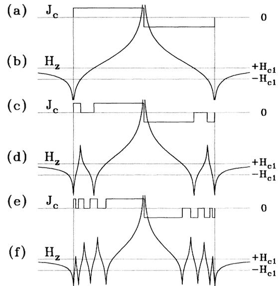
FIG. 5. A possible mechanism of the suppression of the local field at low fields inside a strip discussed in Fig. 4. A starting current distribution (a) produces the field profile (b). Due to the divergence of the field at the edge, the current in the region, where the local field is between  $\pm H_{c1}$ , will be suppressed to zero (c). The current distribution (c) tries to produce the field distribution shown in (d). This process continues (e), (f) leaving many small regions of  $J_c = 0$ .
