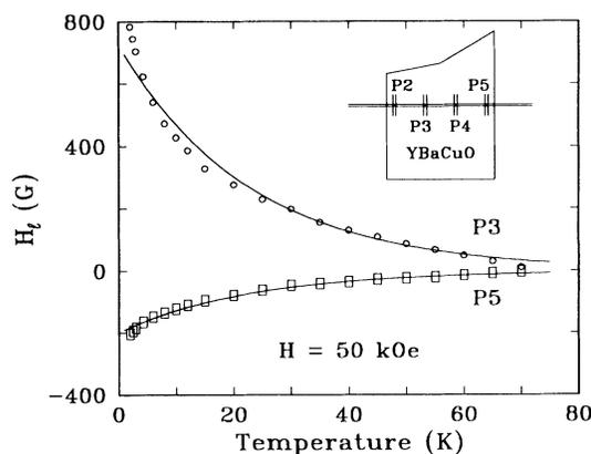
FIG. 1. Temperature dependence of the local field  $H_l$  in the decreasing branch of the hysteresis loop at 50 kOe at two positions near the sample. The solid lines are fits to  $H_l(T) = H_l(0)\exp(-T/T_0)$  with  $T_0 \approx 23$  K. Inset shows locations of four Hall probes.
