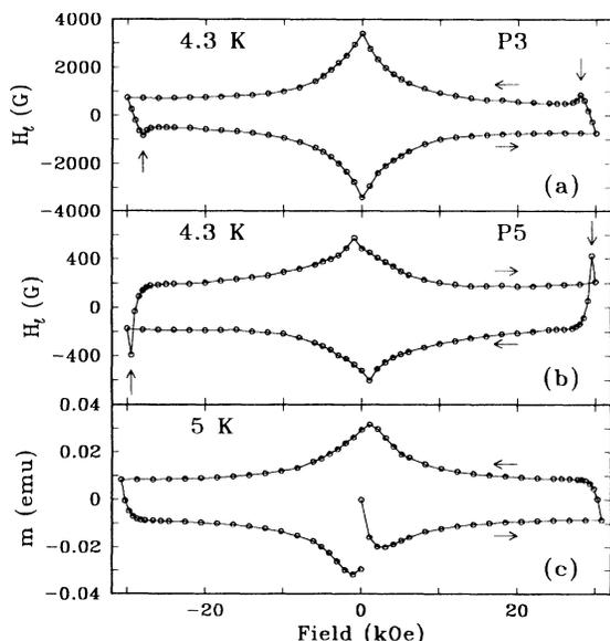
FIG. 2. Local-field hysteresses at low temperatures (a) and (b) measured by two Hall probes of the array and (c)  $M$ - $H$  loop measured by a SQUID on the same crystal. The horizontal arrows show the direction of the external field sweep. Vertical arrows indicate the peaks at the field reversal (PFR).
