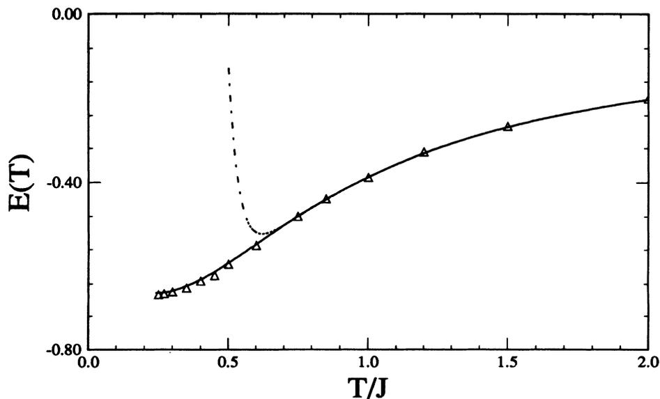
FIG. 1. The internal energy  $E(T)$  vs temperature  $T/J$ . Here the triangle is the data of Makivi and Ding, the dash-dotted line is the direct estimate of the high-temperature series, and the solid line is from our analysis.
