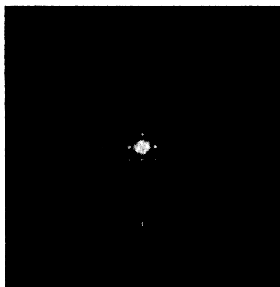
FIG. 13. X-ray diffraction scans of \text{Al}_{60}\text{Cu}_{25}\text{Ru}_{15} annealed at 800^\circ\text{C} for (a) 24 h and (b) 96 h.
