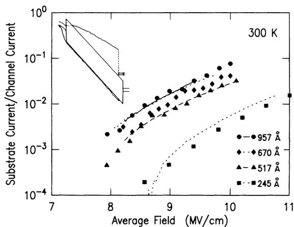
FIG. 3. Measured (curves) and calculated (symbols) values for the ratio of the substrate current to the channel current in *n*-channel FET as a function of oxide field. Results are shown for oxide thicknesses of 245, 517, 670, and 957 Å.
