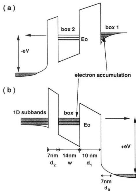
FIG. 1. Band diagram of the asymmetric GaAs- $\text{Al}_x\text{Ga}_{1-x}\text{As}$  double-barrier structure, illustrating the tunneling mechanism. 1D subbands are formed in the contact regions, and 0D states are created in the well. (a) In reverse bias electrons tunnel from the 0D states in the accumulation layer (box 1) into the 0D states in the well (box 2). (b) In forward bias, electrons tunnel from the 1D subbands into the 0D states in the well.
