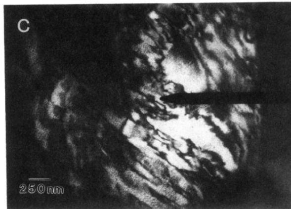
FIG. 6. (a) Electron-diffraction pattern of sample D . Superlattice reflections marked A and B arise from cation ordering along (\bar{1}\bar{1}1) and (1\bar{1}\bar{1}) planes. (b) Dark-field image constructed from superlattice reflection A . (c) Dark-field image of the same area constructed from superlattice reflection B .
