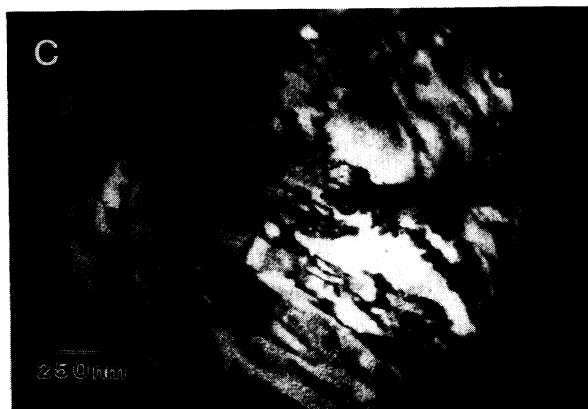
FIG. 6. (a) Electron-diffraction pattern of sample D . Superlattice reflections marked A and B arise from cation ordering along (\bar{1}11) and (1\bar{1}\bar{1}) planes. (b) Dark-field image constructed from superlattice reflection A . (c) Dark-field image of the same area constructed from superlattice reflection B .
