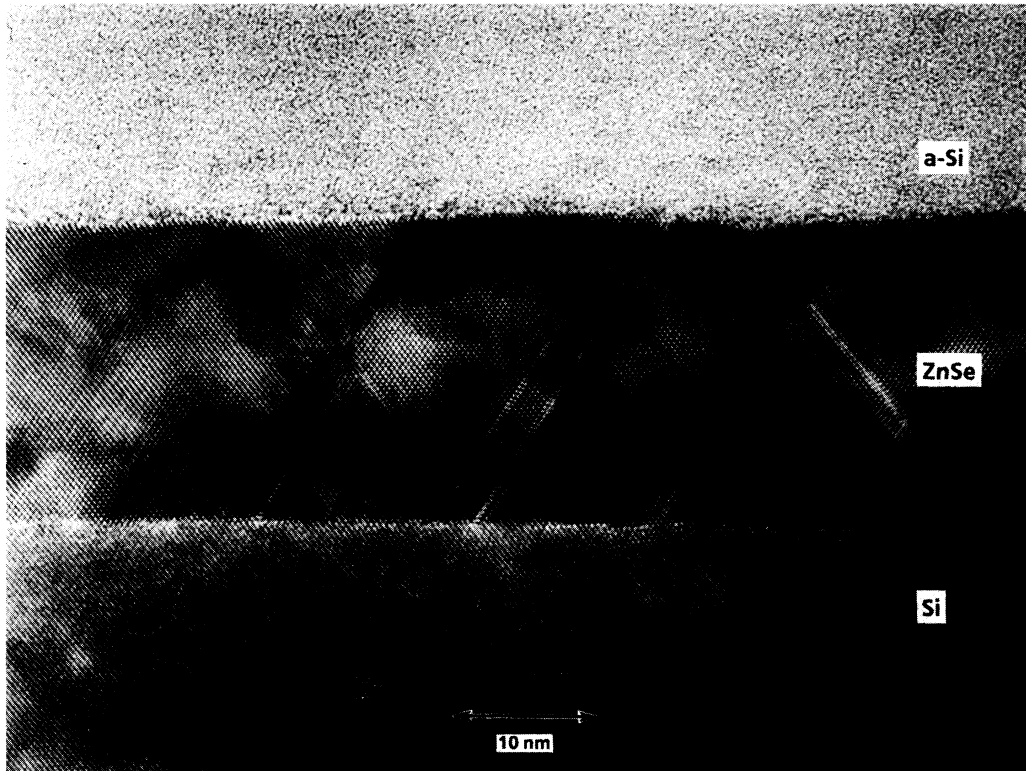
FIG. 5. High-resolution TEM cross section, in a \langle 011 \rangle projection, of a ZnSe film deposited on arsenic-terminated Si(100) at 300 °C. The [100] vector for the substrate is 4° from the interface normal and has a component towards the left of the figure.
