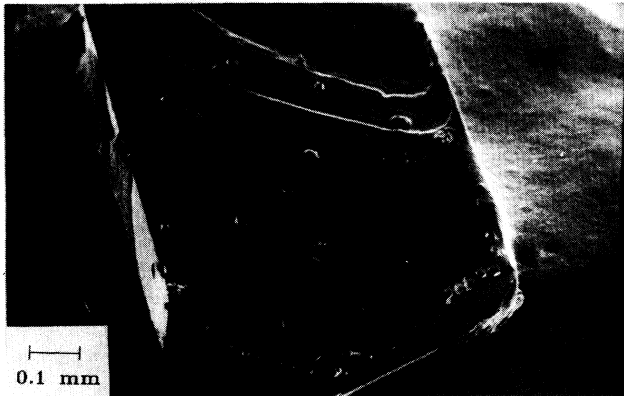
FIG. 2. GaN crystal grown from the solution at N_2 pressure of 1.7 GPa.
