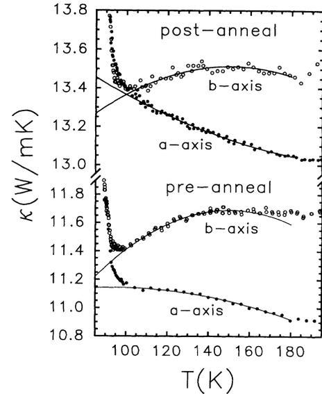
FIG. 2. High-temperature thermal conductivity vs temperature for the untwinned YBCO crystal before and after oxygen anneal. The solid lines represent second-order polynomial fits to the data for  $108 \leq T \leq 170$  K.
