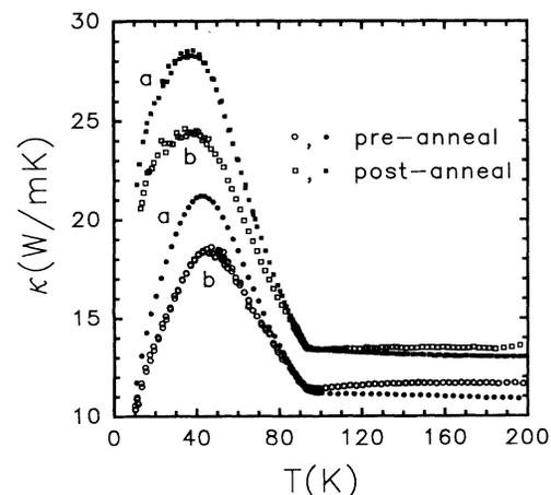
FIG. 1. Low-temperature thermal conductivity vs temperature for the untwinned YBCO crystal before and after oxygen anneal.
