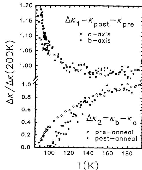
FIG. 3. Difference thermal conductivities vs temperature, calculated from the data in Fig. 2 and normalized to values at 200 K. The upper panel shows  $\Delta\kappa_1 = \kappa(\text{post-anneal}) - \kappa(\text{pre-anneal})$  for the  $a$  and  $b$  axis data. The lower panel shows  $\Delta\kappa_2 = \kappa_b - \kappa_a$ , before and after the oxygen anneal.
