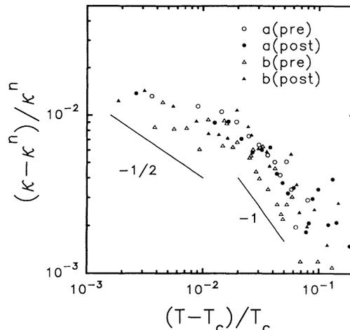
FIG. 4. Normalized fluctuation thermal conductivity,  $(\kappa - \kappa^n)/\kappa^n$ , vs  $(T - T_c)/T_c$  ( $\kappa^n$  is defined by the solid lines in Fig. 2).
