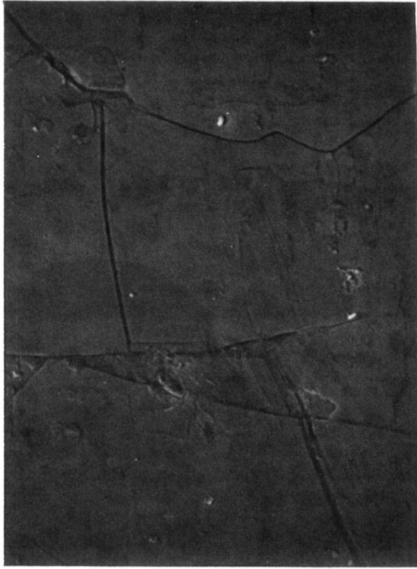
FIG. 3. Surface morphology of the film investigated by scanning electron microscopy.
