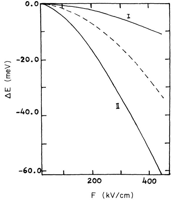
FIG. 2. Comparison of the energy shifts for the bound polaron in a finite QW and in an infinite QW. The solid lines show the results for a finite QW with  $L = 34$  Å (I) and  $L = 100$  Å (II). The dashed line shows results for an infinite QW with  $L = 100$  Å.
