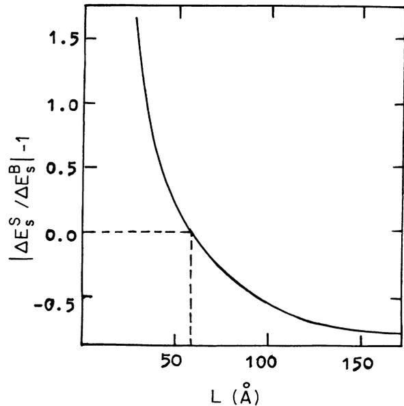
FIG. 5. Plot of the ratio  $|\Delta E_s^S / \Delta E_s^B| - 1$  vs the well thickness.
