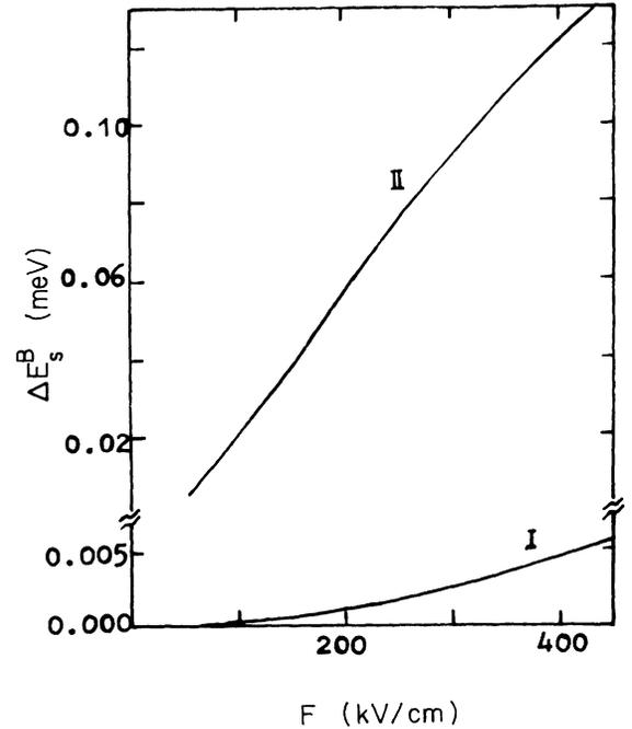
FIG. 3. The correction of LO-mode effect to the energy shift of the bound polaron vs the electric field in a finite QW with  $L = 34$  Å (I) and  $L = 100$  Å (II).
