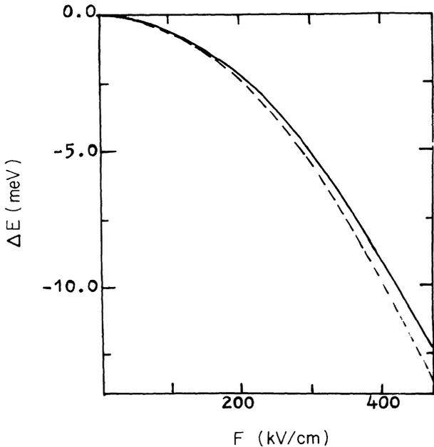
FIG. 1. The energy shifts vs the electric field for an electron in a finite QW with  $L = 34$  Å. The solid line represents results for the well with an on-center impurity and the dashed line those for the well without any impurity.
